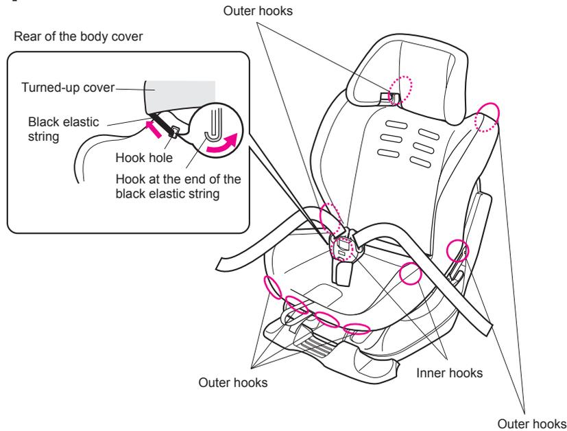
**2** Move up the headrest and release the 2 hooks and 2 fastener tapes of the headrest.
