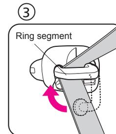
Turn the ring segment upward to lock.
