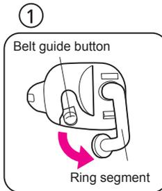
While pressing the belt guide button, turn the ring segment downward to release.
